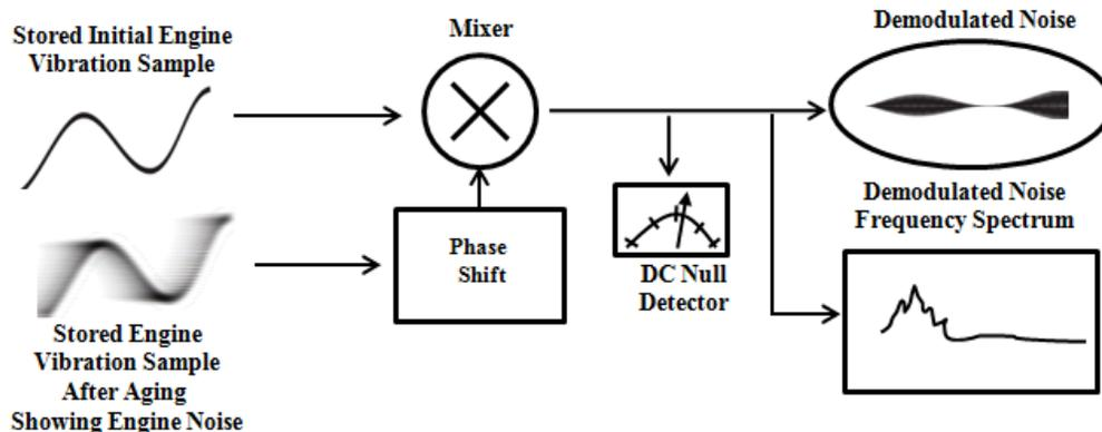
Figure 1 - Active autocorrelation measurement noise demodulation detection
