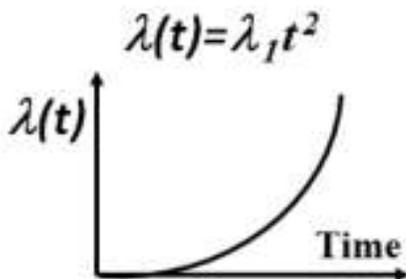
Figure 2 Power law fit to the Wearout portion of the bathtub curve.
