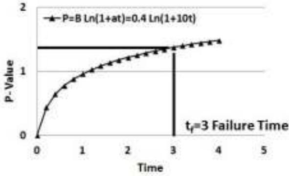
**Figure 3** Log time aging with parametric threshold  $t_f$
