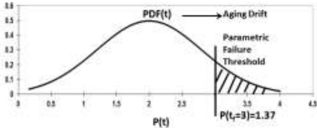
**Figure 4** PDF failure portion that drifted past the parametric threshold
