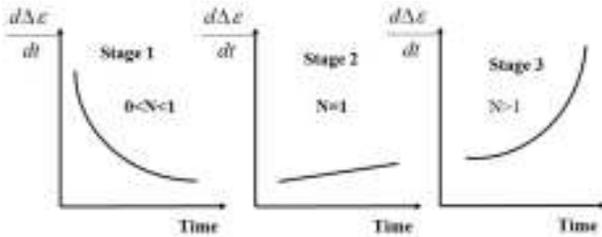
Figure 6 Creep rate power law model for each creep stage similar to the bathtubcurve in Figure 1
