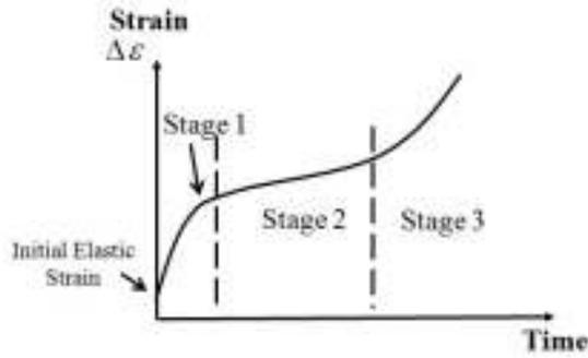
Figure 5 Creep curve with all three stages
