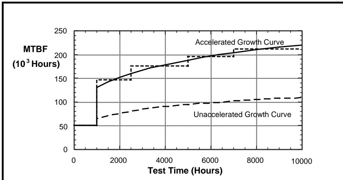
**Figure 9** Accelerated and Unaccelerated Reliability Growth Curve (Reproduced from Ref. 10).
