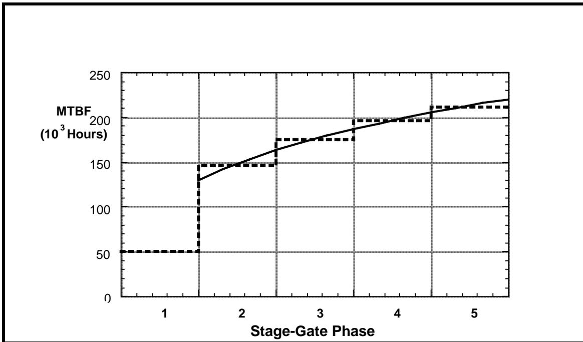
**Figure 9** Mapped Stage-Gate Accelerated Reliability Growth Curve of Figure 8
