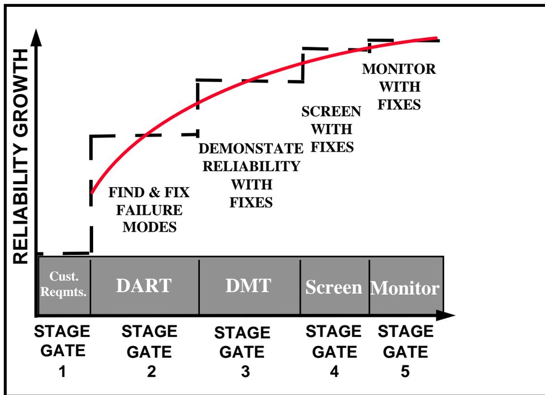
Figure 3 Stage-Gate Accelerated Reliability Growth Model
