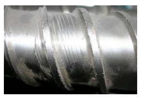
*V*=removed volume of the softer material, *P*=normal load (lbs), *L* is the sliding distance (feet), *H*=hardness of the softer material in psi, wear volume *V*=*AD* where *A* is the area and *D* is the depth of the removed. Then writing L=v t for two sliding surfaces rubbing against each other at a constant velocity v,  $\tau$  failure time.
